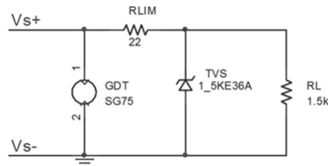
Fig. 5 Protection circuit with  $R_L$  load resistor
