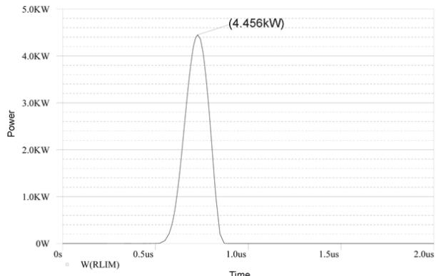
Fig. 10 Dissipated power in the limiting resistor
