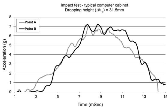
Fig. 3 An example of measured acceleration at impact
