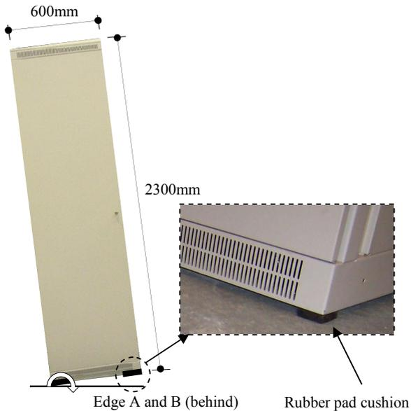
Fig. 2 Test setup for the physical full-scale experiments
