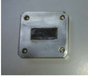
Fig. 2 (a) X-Band sample holder and RHCNTs sample
