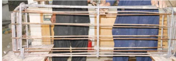
Fig. 3 Steel skeletons for beam specimens
