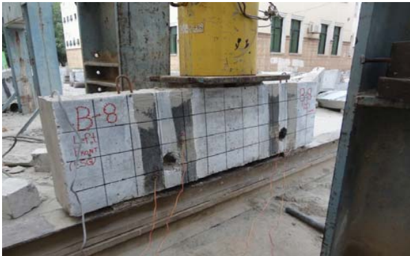
Fig. 5 Loading arrangement for beam testing
