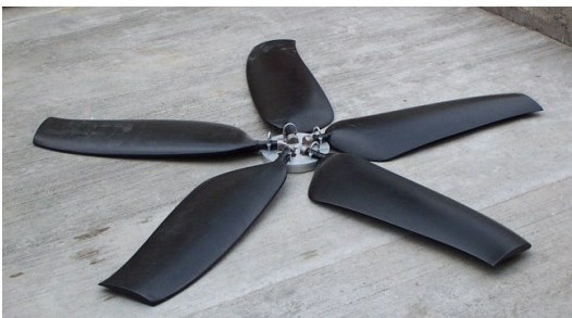
Fig. 6 A 1.618m Propeller fan wheel with 5 blades
