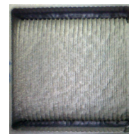
Fig. 4 Sample pocket milled surface
