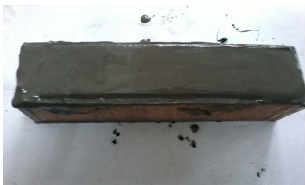
Fig. 2 CNT/Cement mixture in wooden mould
