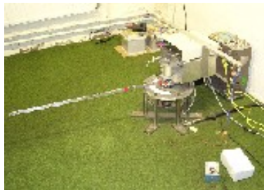
Fig. 1 The laboratory-scale single-link flexible manipulator
