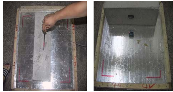
Fig. 8 Experiment of Measurement of Electric Waves Attenuation
