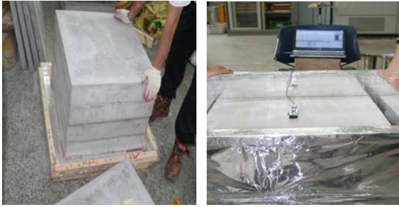
Fig. 6 Permeability Experiment in Vertical Direction
