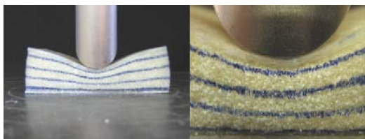
Fig 3 indentation in sandwich beam with PU core
