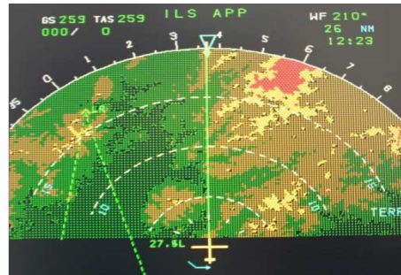
Fig. 9 Terrain map displayed on ND
