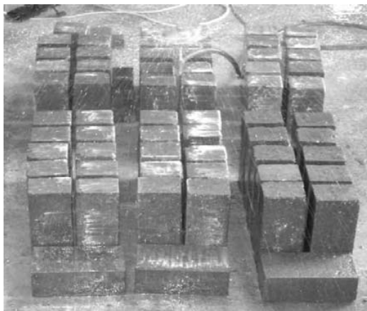
Fig.3 The curing of paving block samples
