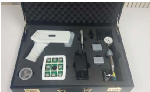
Fig. 9 Picture of the portable ultrasonic leak detector
