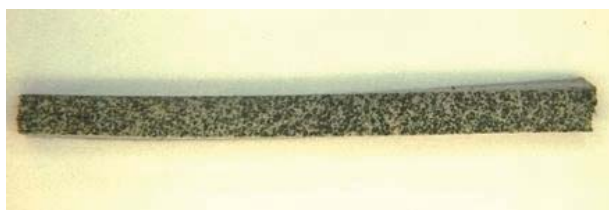
Fig. 3 A strip of the epoxy modified with rubber sample after 2 months exposure to deionized water at 80°C and complete drying
