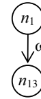
Fig. 2. The control flow graph of the function find reduced to the entry node and the exit node
