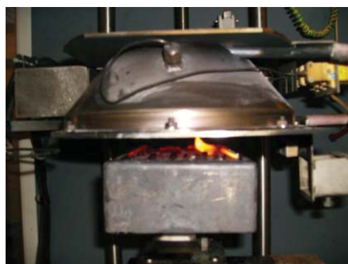
Fig. 8 Detail of the flame extinction process for composites 2: 1 and 1:1
