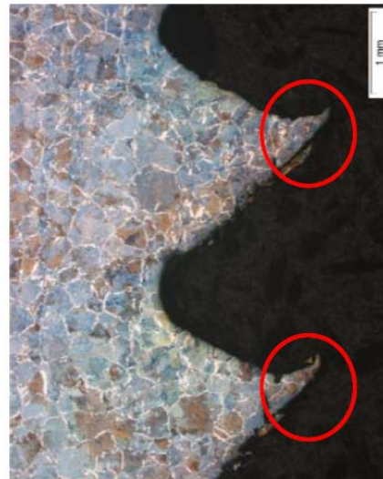
Fig. 10 The presence of a sharp edge in the peaks of the threads of the seat of the fracture pin 1
