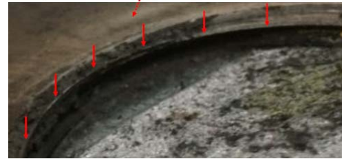
Fig. 8 Presence of sharp edge (sharp corners) in the peaks of the threads of the seat of the fracture pin 1
