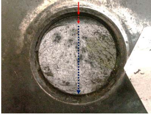
Fig. 7 The visual inspection of the fracture shows: region of beginning of the fatigue crack (red arrow); beach marks: beginning and propagation of fatigue crack by unidirectional flexion (red dotted arrow); and radial marks: region of instantaneous fracture and final of brittle fracture (blue dotted arrow)
