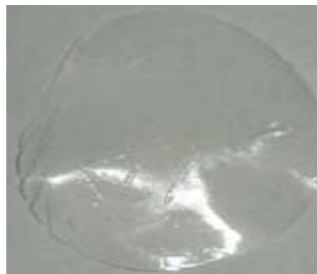
Fig. 1 PVDF pure sample prepared by melt at 200 °C under 300 bar
