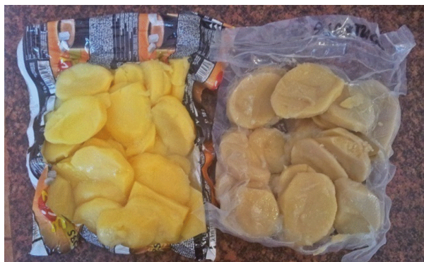
Fig. 5 The influence of packaging material on the potatoes (control) samples color after 4 storage months
