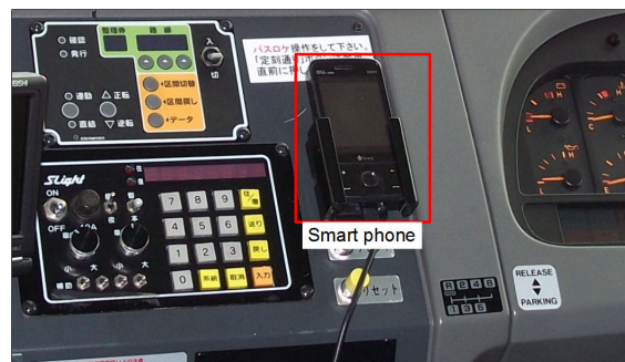
Fig. 6. Installed smart phone in a bus.
