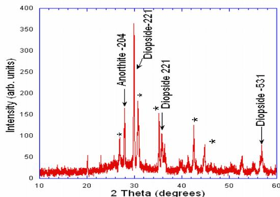
Fig. 2 XRD pattern of glass-ceramics GD12Pb. Stars (\*) represent Bragg's peaks of the New Pb-rich phase (NPb), while main peaks for diopside and anorthite are assigned with  $hkl$  Miller indices. Note the coarse background at  $2\theta$  around  $30^\circ$  which is a signature of the glass-matrix.
