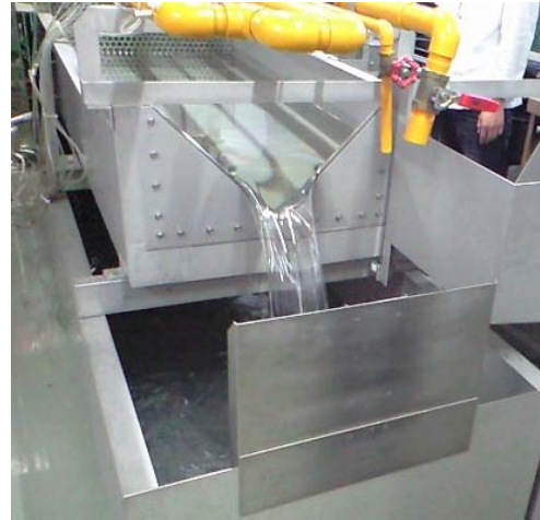
Fig. 2 Regular triangular weir of 320 mm side length
