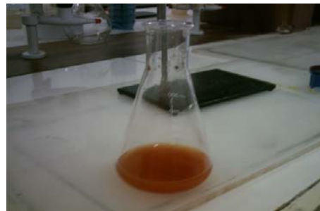
Fig. 6 Pinkish end point colour after titration
