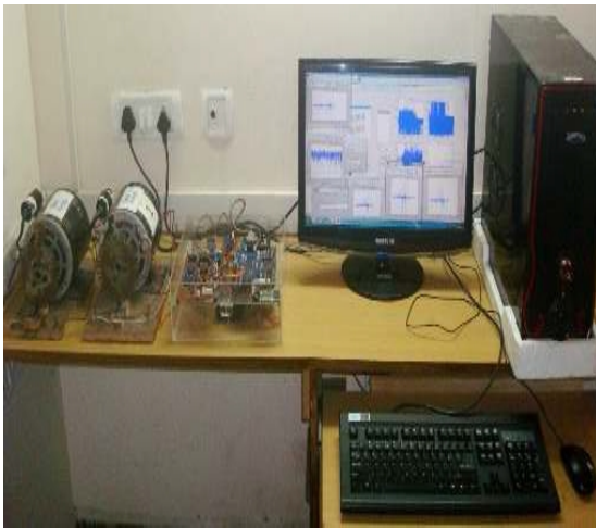
Fig. 3 Experimental setup using healthy and unhealthy motor
