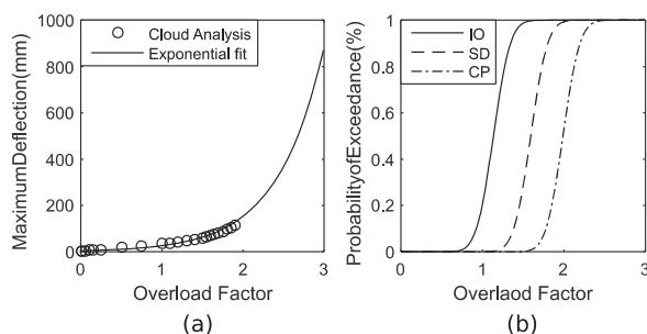
Fig. 6 (a) The median function and (b) the fragility curves for the three limit states
