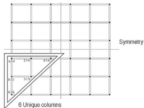
Fig. 3 Structure's symmetry and the considered columns
