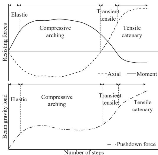
Fig. 1 The three stages of nonlinear beam behavior
