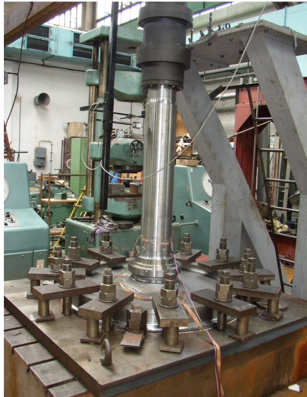
Fig. 20 Experiments on a massive machine for the dynamic testing of railroad axles (see reference [1])
