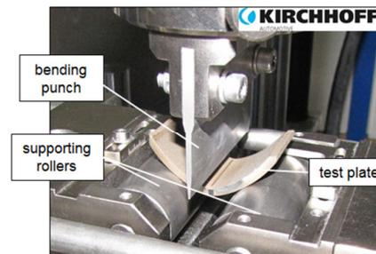
Fig. 13 Experimental setup of the three-point bending test
