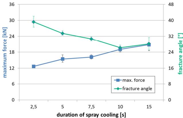
Fig. 14 Results of the three-point bending test
