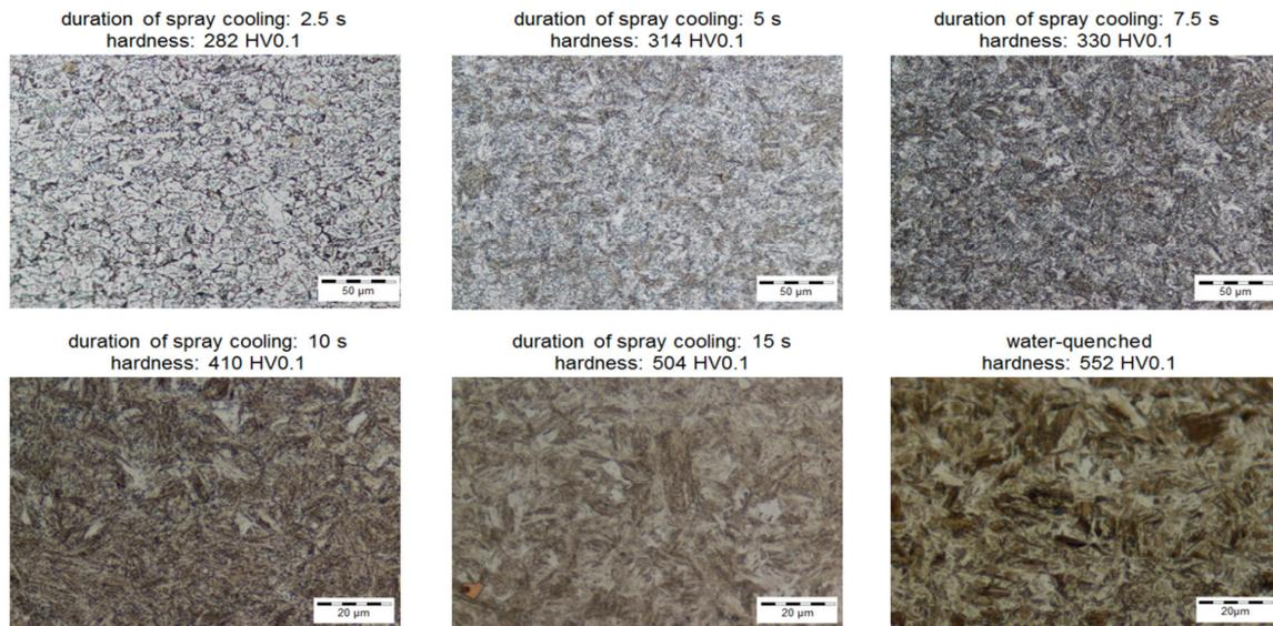
Fig. 15 Microstructure of samples with different cooling duration
