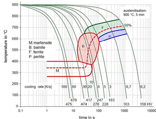
Fig. 1 Time-temperature transformation (TTT) diagram of 22MnB5 [6]
