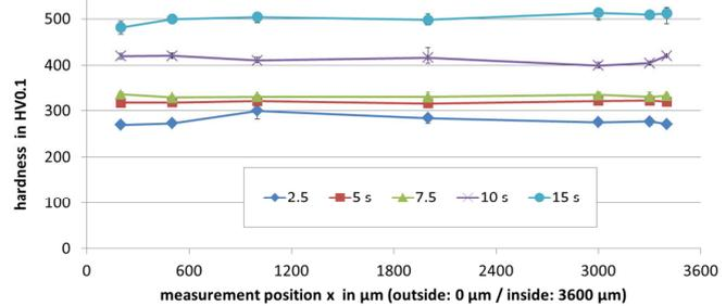
Fig. 12 Hardness measured across the wall thickness
