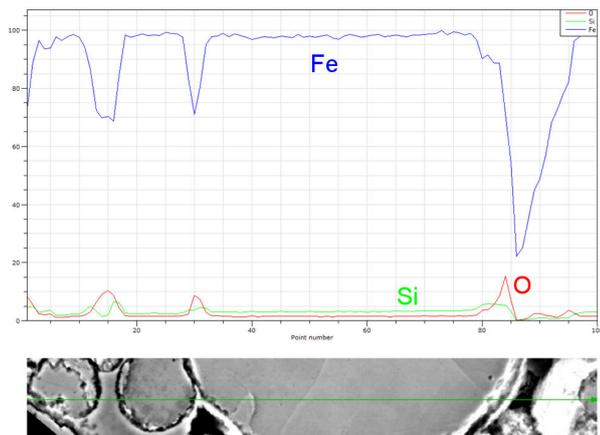
Fig. 10 EDS line analysis of FeSi-ferrite inter-particle connections
