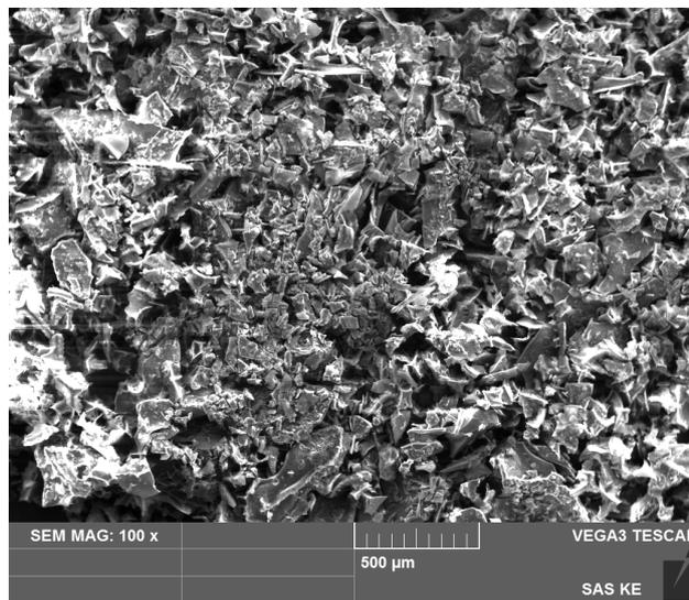
Fig. 3 SEM morphology of synthesized MnZn ferrite
