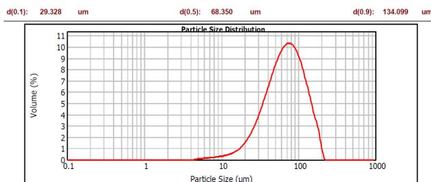
Fig. 6 Particle size distribution of the Fe-3Si powder
