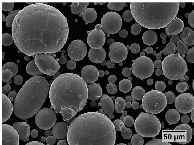
Fig. 5 SEM morphology of Fe-3Si powder alloy
