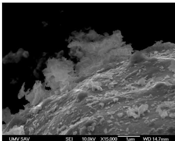
Fig. 8 Surface of FeSi particle with ferrite nano-particles
