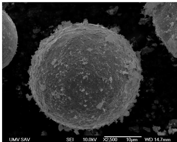
Fig. 7 FeSi powder particle covered by ferrite nano-particles
