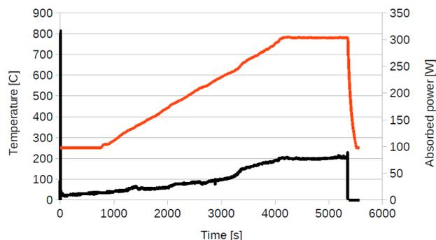
Fig. 2 Microwave sintering time-temperature and absorbed energy profile
