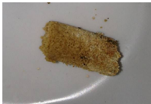
Fig. 9 Sintering of composite catalyst bed after test
