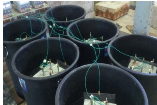
Fig. 2 Accelerated corrosion apparatus for column elements
