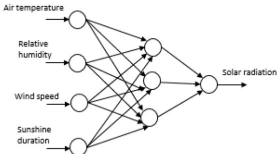
Fig. 2 The fully connected MLP used in the reference estimation system
