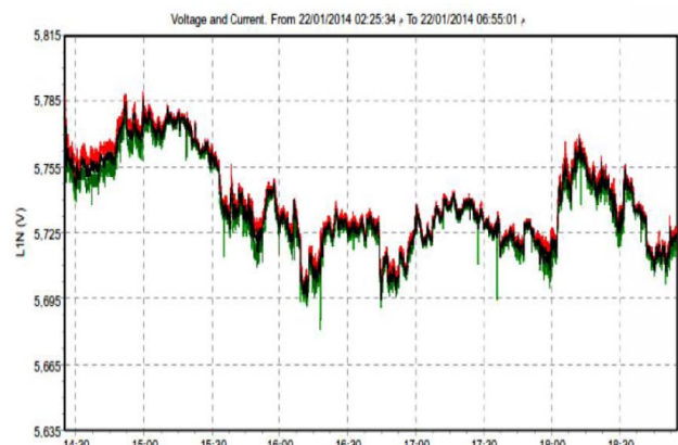
Fig. 4 Voltage variation in Al-Nasim Dairy
