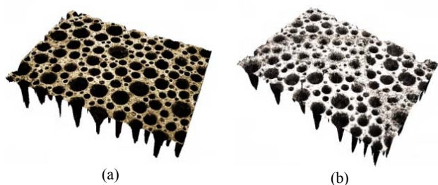
Fig. 5 3D confocal laser micrographs before (a) and after (b) the six immersions
