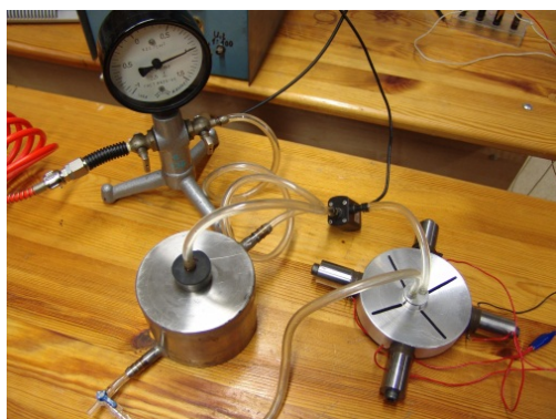
Fig. 20 The experimental setup for algae ultrasonication by system shown in Fig. 3b
