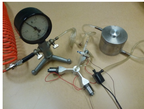
Fig. 16 The experimental setup for algae ultrasonication by system shown in Fig. 3a
