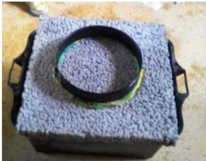
Fig. 3 Pervious concrete permeability test setup [13]
