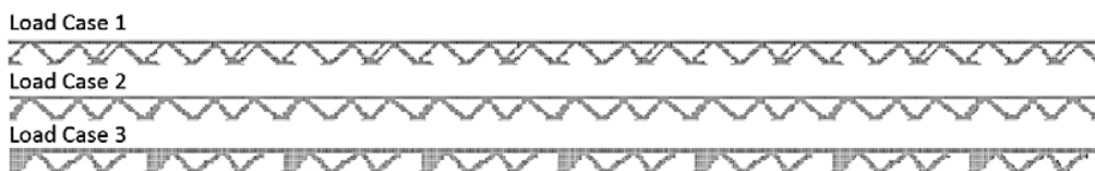
Fig. 7 Topology optimization results of three load cases
