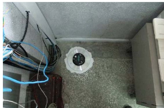
Fig. 1 A seismometer was mounted on the ground of the first floor of the school building in the first stage
