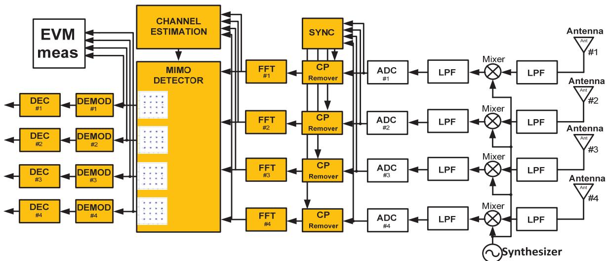
Fig. 3 The 4x4 MIMO LTE DL PHY layer architecture: (a) distributed and (b) co-located technique
