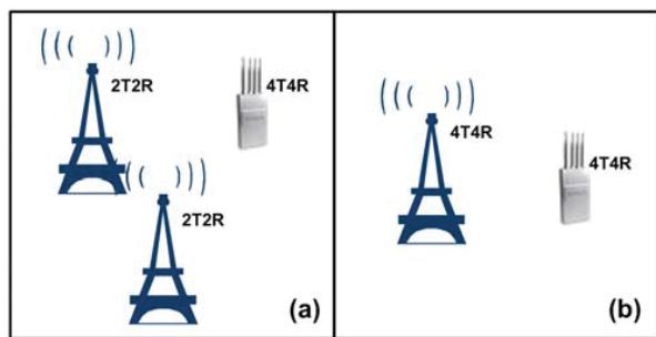
Fig. 1 (a) Distributed and (b) co-located 4x4 MIMO system in actual system realization
