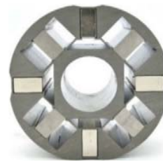
Fig. 17 Manufacture version of VF-PMSM rotor
