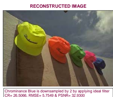
Fig. 2 Reconstructed Image in case of downsampling the Cb by 2
