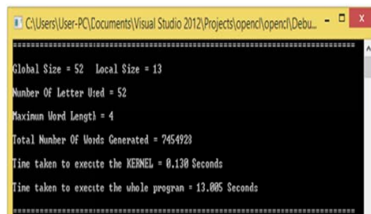
Fig. 2 (b) Time taken by the Kernel and the whole program with Work Item size = 13 and Work Group size = 4
