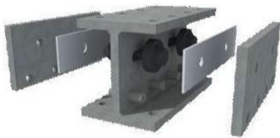
Fig. 8 Shear friction damper
