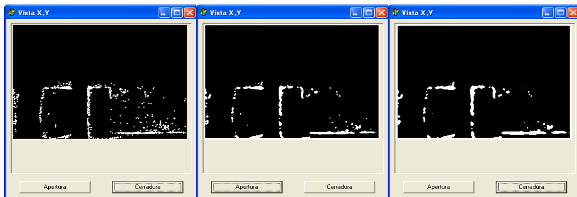
Fig. 16 The X-Y view. We apply the opening operation to deleted isolated flies, next we apply the closing operation to delineate the objects
