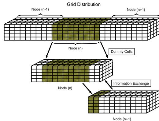
Fig. 3 Schematic of decomposed domain method using dummy cells
