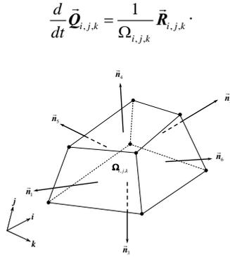
Fig. 1 Control volume and associated interface unit normal vectors for a structured grid
