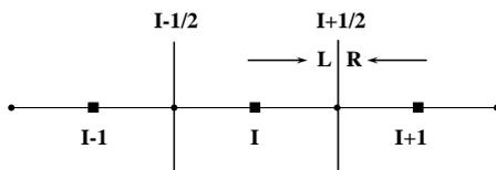
Fig. 2 Left and right state at cell interface
