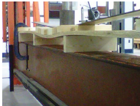
Fig. 9 The uniformly distributed load is mimicked by a series of wood blocks under the steel bar
