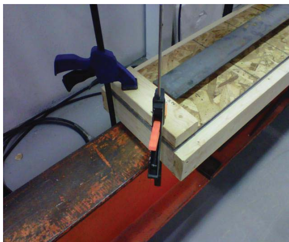
Fig. 10 C clamps were put in place to hold the end supports from lifting
