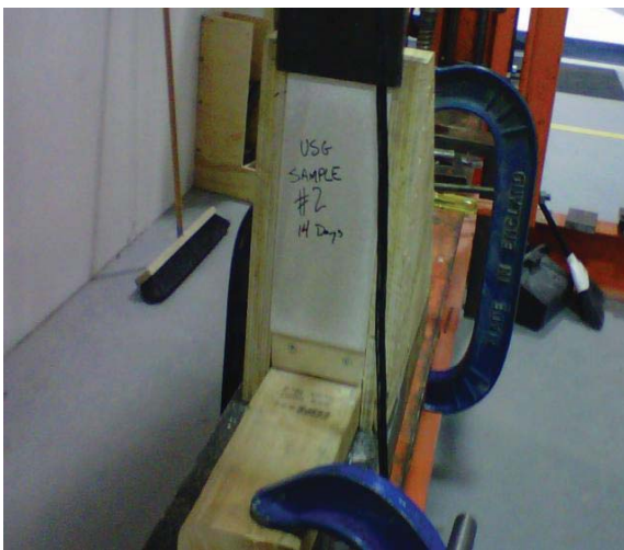
Fig. 2 The overlay layer was pushed down in order to measure the shear bond strength between OSB and the overlay
