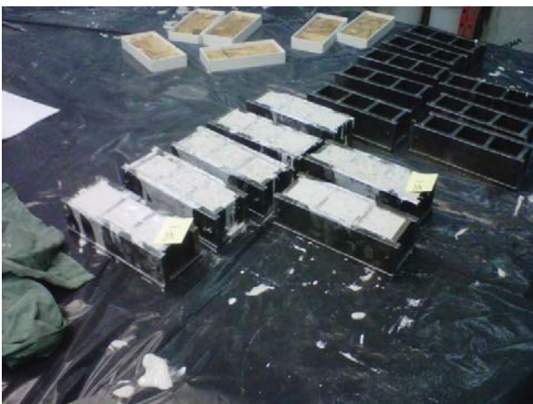
Fig. 3 Standard Cube and Shear Bond Specimen Molds
