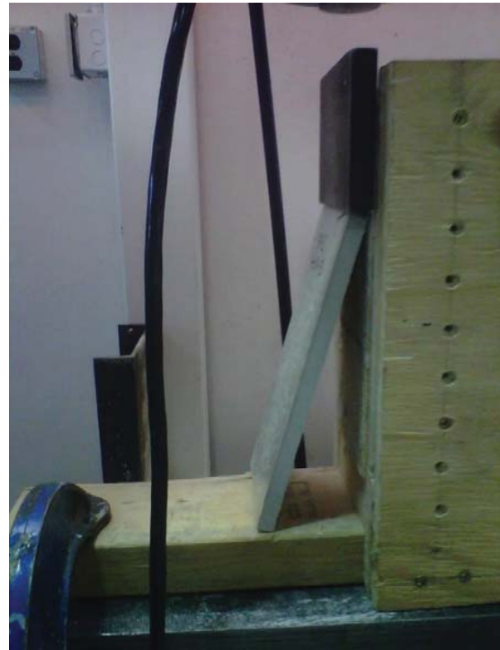
Fig. 4 The overlay separated from OSB due to slip failure
