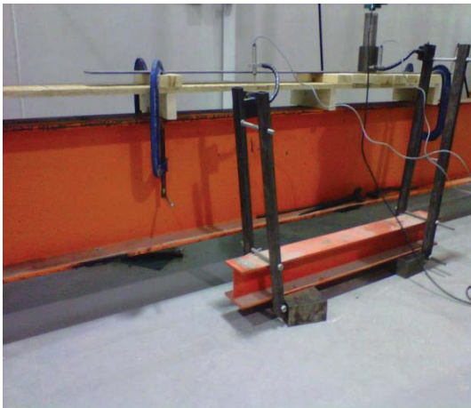
Fig. 7 The Side Span Loaded by the Distributed Load System
