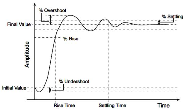
Fig. 2 Signal Constraints for a unit step input
