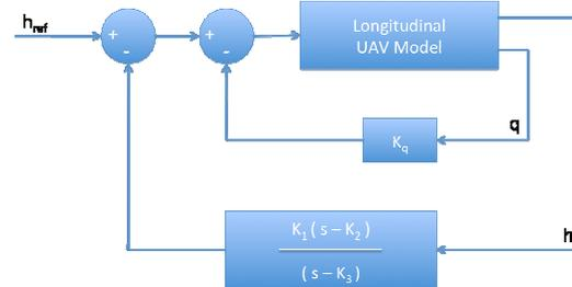
Fig. 1 Altitude-Acquire & Hold Phase Lead Compensator
