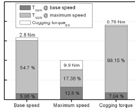
Fig. 7 Characteristics in optimal model of each response
