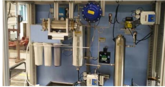
Fig. 3 Core holder apparatus
