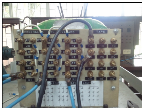
Fig. 5 Connection board of the motor under test
