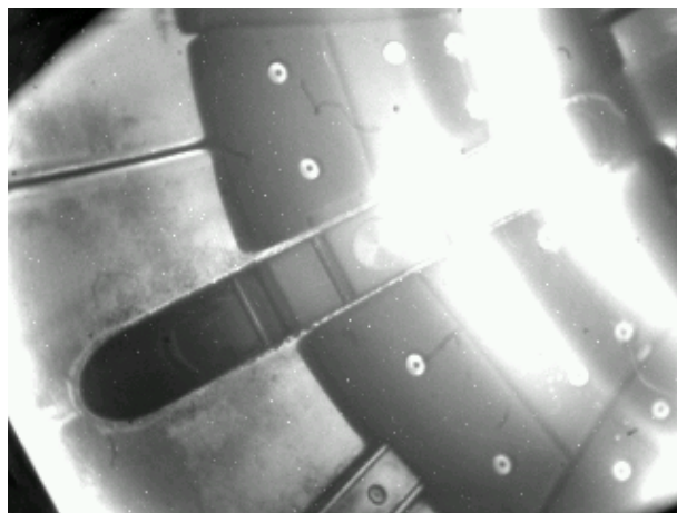
Fig. 5 Observation of the divertor leg traces using the slow CCD camera on the COMPASS tokamak in the shot #3329. Exposure time is 100 ms, starting at 1162 ms
